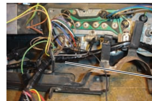
Circuit Node #2, at the center lower clip of the Instrument Panel
