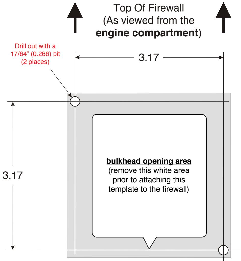
The only firewall modification needed with this new kit is to drill 2 new 0.266 mounting holes. The stock opening in the firewall is already the proper size for the new bulkhead assembly to fit through. This template can be affixed directly to the firewall or it can be applied to a stiff piece of cardboard or thin plastic, then mounted to the firewall. Be sure to clean any wax, grease, or oil from the area so that the template will stick.
